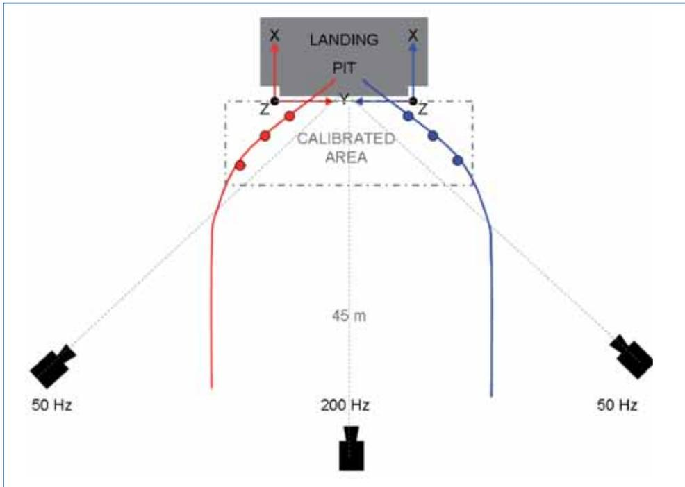
Figure 1: Camera positions, co-ordinate system and the multi phase calibration area used in the high jump at the 2005 IAAF World Championships in Athletics
