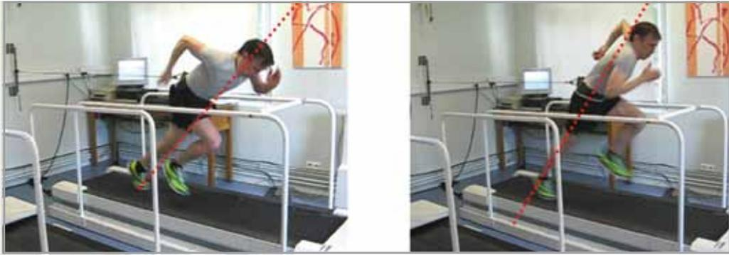
Figure 2: The sprint instrumented treadmill
