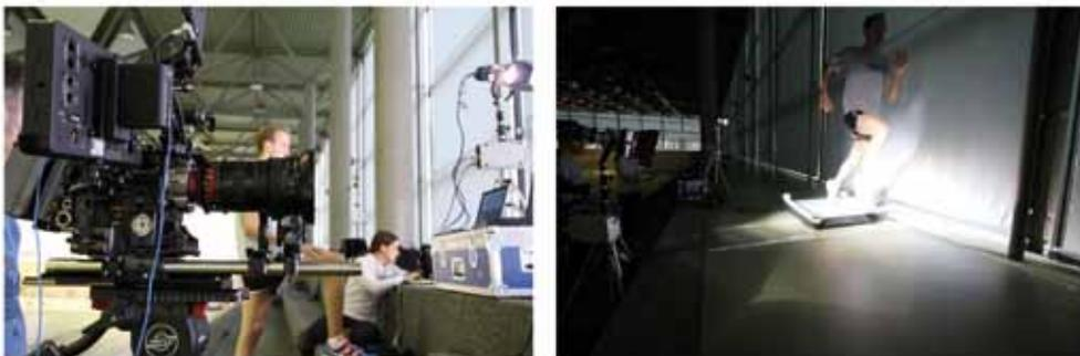
Figure 8: Red high-speed camera (left) and measurement setup with Kistler force plate and Optojump (right)
