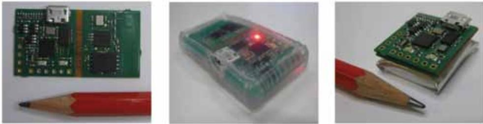
Figure 3: PARTwear unfolded without casing (left), with silicone casing (center) and folded (right)
