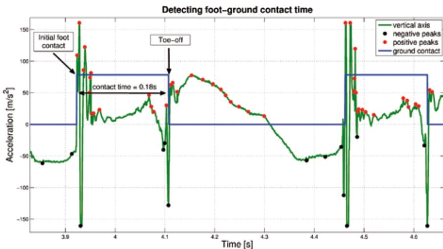
Figure 6: Detecting foot-ground contact time using a peak detection algorithm
