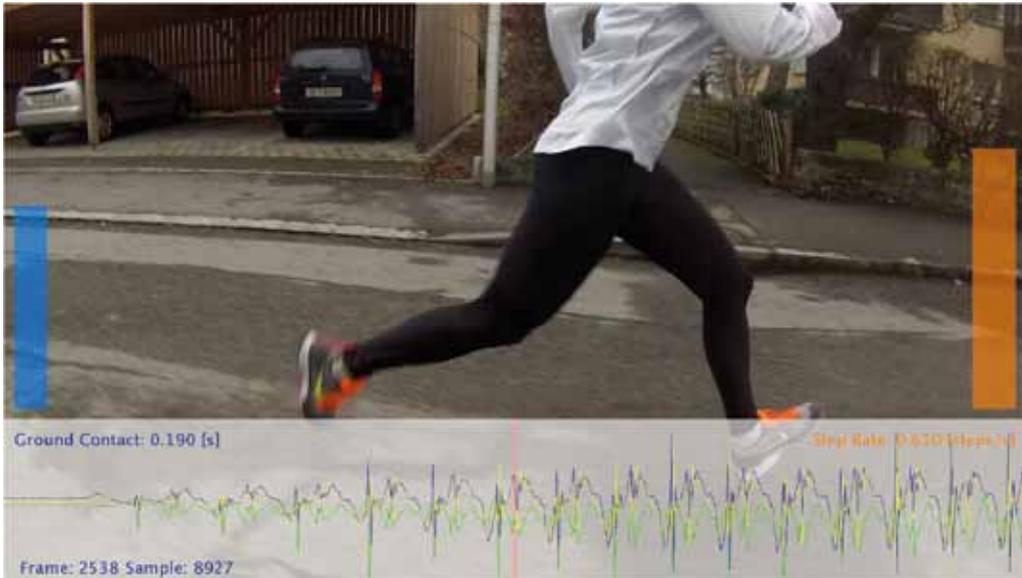
Figure 7: Acceleration data of each sensor axis and the computed foot-ground contact time as well as the step rate are displayed in a video file
