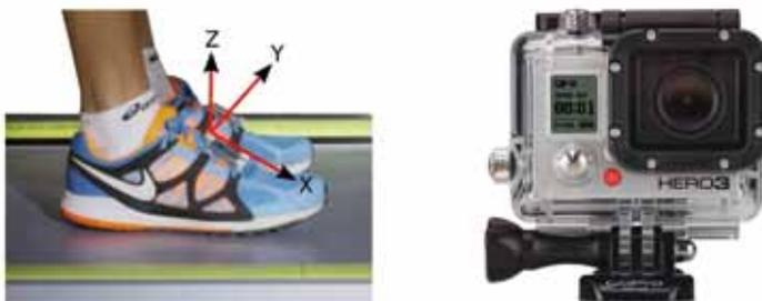
Figure 4: PARTwear sensor attached to the right foot (Positive directions of the three acceleration axes are superimposed. (left), and GoPro HERO3<sup>®</sup> camera (right))
