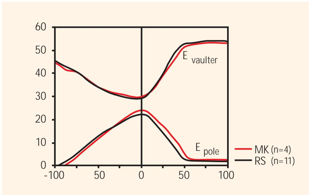
Figure 3: Comparison of the mean total mechanical energy and mean strain energy of the pole of two elite pole vaulters (training session). The x-axis is normalised as follows: -100% up to 0% represent the phase between the beginning of the vault and the maximum pole bend position; 0% up to 100% represent the phase between the maximum pole bend position and the instant of maximum centre of mass height.
