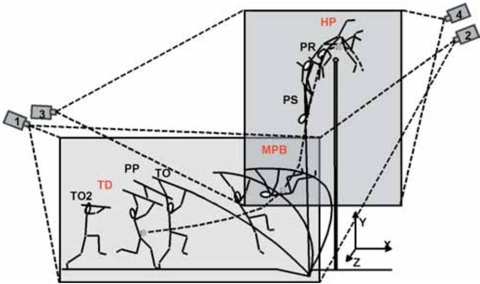
Figure 2: Common camera set-up and calibration for a 3-D kinematic analysis of the pole vault (TO2=take off 2, end of second last ground contact, TD=beginning of last ground contact, PP=pole plant, TO=end of last ground contact, MPB=maximum pole bend, PS=pole straight, PR=pole release, HP=highest point of centre of mass).
