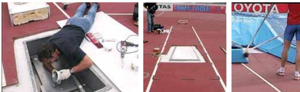
Figure 2: Set up of dynamometric vault box.
